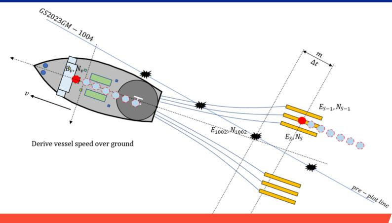
The software functionality offer our data analysts the tools to identify and eliminate positioning errors to improve the integrity of the associated seismic trace data. Horizontal and vertical positioning errors in the seismic data will only propagate into decisions made from this data such as the selection of a proposal well location. By automating the workflows and QA/QC procedures means these services are offered to you in a time and cost effective manner.
